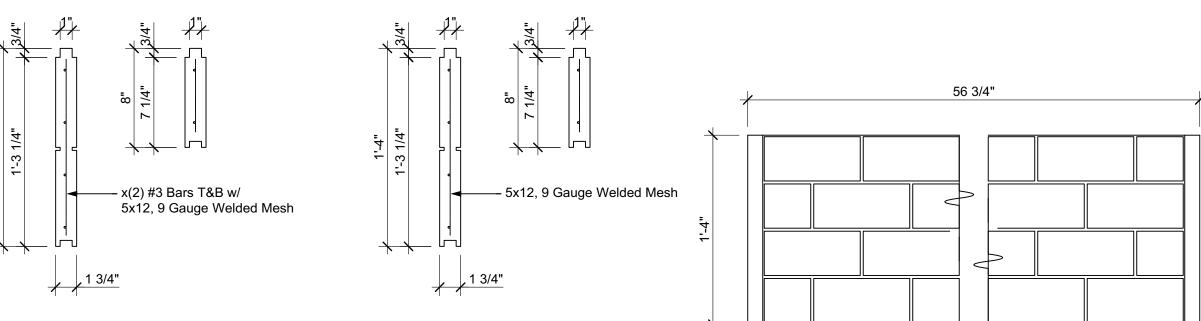
STANDARD PANEL **END PANEL - SECTION MID-WALL PANEL - SECTION**
